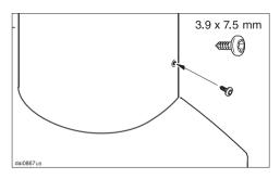
Secure the chimney to the motor assembly and lower retaining plate with the remaining screws.
